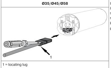
Insert the **dead** connecting cable into the drive head until the locating lug clicks into place in the drive. If necessary, use a suitable flathead screwdriver to assist with insertion. Set the screwdriver into one of the two plug grooves provided for this purpose.
